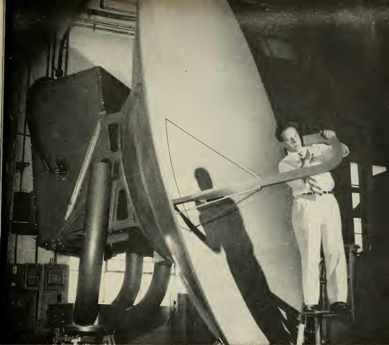
Twelve-foot diameter dish of WSR-57 "Stormfinder" radar. System operates at S band, has 250-mile range, 500 Kw output.
