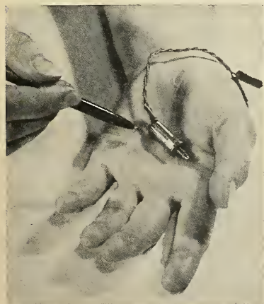
SUBMINIATURE electro-hydraulic valve cycles in a few thousandths of a second and can be actuated by an electromagnet.
