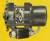
Type: D-932 DC Motor. Weight: With radio noise filter — 13 lbs., without same — 12,4 lbs. Terminal voltage: 27.5 DC plus or minus 1.5 volts. Load: From .5 hp minimum to 2.6 hp maximum. Speed: Continuous at 12,000 rpm, plus or minus .005%. Speed Control: By frequency regulator supplying control field. Meets Military Specification MIL-M-8609 (ASG).
