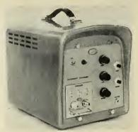
direct pressure measurements is being introduced by Wianco Engineering Co. The portable, compact unit has an overall accuracy of  $\pm 0.05\%$  of full-scale ranges of
