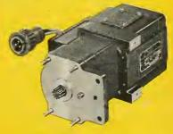
Type: D-927 DC Motor. Weight: 7.25 lbs. with 2-circuit noise filter for ungrounded systems, Weight of filter: 1 lb. Terminal voltage: 27 volts, 18 amps. Load: 0.5 hp. Speed: Continuous at 9900 rpm. Meets Military Specification MIL-8609.
