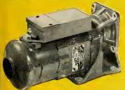
Type: D-751 DC Motor. Weight: 20 lbs. Duty Cycle: 5.2 hp at 2100 rpm (intermittent) on 26 volts DC; 3.5 hp at 2200 rpm (continuous) on 26 volts DC. Meets Military Specification MIL-M-8609.
