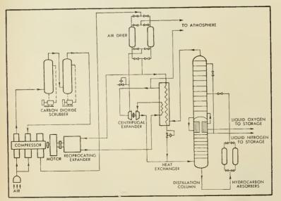
Flow diagram of 75 T/D LOX Generator. It's said to cut big quantity production rates to about .7¢ per pound of LOX and liquid nitrogen. Designed to run by electric power.
