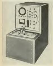
Use of a long persistent oscilloscope pro-vides display of error signal, and noise due to contact resistance over frequency range of 0 to 100,000 cycles. Individual wire commutation may be shown. Mag-netic clamping allows rapid set-up and diagramet of perturbative teralignment of test potentiometers.
