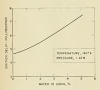
Table showing overall effect of water in UDMH on ignition delay with IRFNA.
