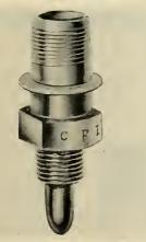
n a stainless steel body has been inroduced by Control Products, Inc. The witch operates in ambient temperatures from  $-65^{\circ}$ F to 700°F, has an electric rating of 2 amps and is resistive at either 28V dc or 115V ac. Length over AN connector is 5/16" and it is designed to neet environmental, shock and vibration requirements of MIL-E-5272A.
