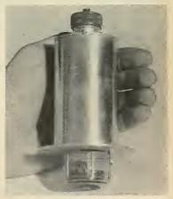
tems, programming devices and explosive element initiation. The unit provides for a settable time delay between 0.3 and 10 seconds, with an accuracy of  $\pm 5\%$ , and output energy in excess of 35,000 ergs. Temperature ambients from  $-70^{\circ}$ F to  $165^{\circ}$ F and accelerations up to 100 g's have no effect on the device, which is termed the PM.47 termed the PM-47.
