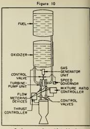
Rocket powerplant with turbine/pump-unit including automatic thrust and mixture ratio control.
