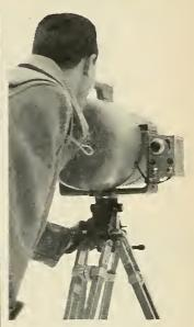
A Barnes OptiTherm Radiometer is essential for precise, quantitative infrared radiation studies of military targets or backgrounds. These instruments are so rugged and stable that they have been successfully used in airborne as well as field studies. Barnes equipment was the overwhelming choice of a majority of the participating groups in the pioneering ARDC Infrared Measuring Program.
