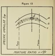
Automatic control of  $P_e = constant$  and mixture ratio = constant. a to c are curves of three different  $P_e$  values as parameters. S = area covers the tolerance for an acceptance test.
