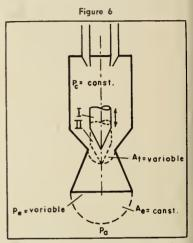
Parameters of a variable expansion nozzle.
