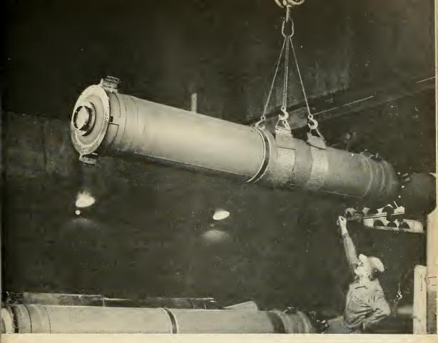
HONEST JOHN, complete except for propellant, worhead and fins, is built of steel by ALCO under prime contract.
