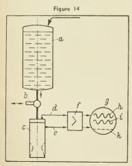
Test arrangement for the stability investigation of a mono-propellant pressurized system, (a) propellant tank (b) piston pulser to generate a harmonic disturbance (c) combustion chamber (d) injection pressure Pr (e) chamber pressure Pc (f) amplifier (g) oscillograph (h) P, as the input variable (i) Pc as the output variable (k) time mark.
