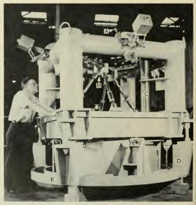
VANGUARD launching and static test platform, manufactured by Loewy-Hydropress, as it awaited shipment to Patrick AFB, where it has been installed for some weeks. (A) Pullaway pickup points on which the rocket rests, (B) the tripod which supports the engine, (C) pipe to carry exhaust to flame deflector, (D) one of four load cells to weigh rocket, fuel, measure thrust and similar functions, and (E) weighing ring for the entire unit. missiles and rockets
