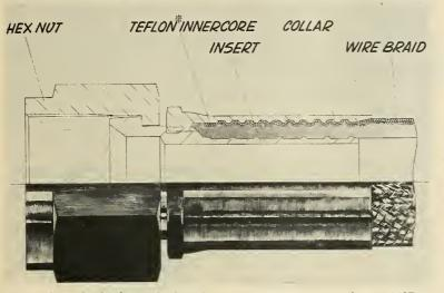
As shown in the figure, the hose is retained between an insert and a collar. Originally a loose fit over the wire braid, the collar diameter is reduced a predetermined amount by radial pressure ap-plied progressively along its length in a rotary hydroforming machine. The plastic innercore and the braid are worked forward toward the hex nut, resulting in a
