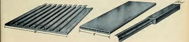
**INTEGRALLY STIFFENED SKIN PANEL** is produced in extra wide widths on heavy presses. Combination of skin and stiffeners in large panels minimizes machining, simplifies assembly, improves performance of aircraft, missiles, and military vehicles. **DECK COOLING PANEL** for aircraft carrier is extruded on heavy presses. Light-weight, water-tight aluminum panels circulate water to offset intense heat generated against deck in jet aircraft operations.
