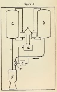
Mixture ratio control system or the sounding rocket VIKING. (a) oxidizer tank (b) fuel tank (c) differential pressure sensor (d) mixture radio controller (e) actuator (f) control valve (g) combustion chamber.
