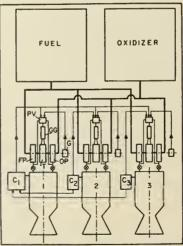
High thrust powerplant applying three combined rocket units. The master controller  $C_{\perp}$ of unit I mixes the signals received from the other controllers  $C_{2}$  and  $C_{3}$  and compensates for the deviation according to the thrust set valve. Separate governor control loops are required to maintain stable conditions during starting transient. (PV = prop. valve; GG = gas generator; T = turbine; FP = fuel pump; OP = oxidizer pump; G = governor.)
