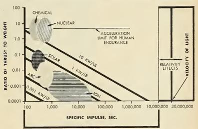
Ratio of thrust to weight versus specific impulse, sec., of different propulsion systems.
