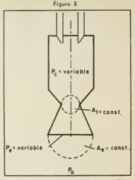
Parameters of a fixed expansion nozzle.
