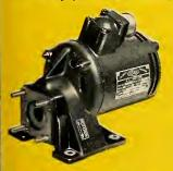
Type: D-899 400 cycle 3 phase AC Motor. Weight: 11.25 lbs. Volts: 200 volts. Vodt: 2.75 hp continuous output. RPM: 3140 rpm output at gear box. Power facter: 83%. Overall efficiency: 76% forentire unit. Meets Military Specification MIL-M-7969A (ASG).
