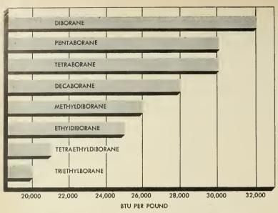
Comparison of heat output from various types of borane used as rocket propellants.
