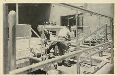
Mechanics Walter Pressir and J. W. Stewart set water-flow control valves on Rocketdyne's high flow bench used to test fuel control components in large liquid fuel rocket engines.
