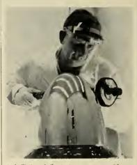
A ballistic missile test nose cone, with one of the smoothest surfaces created by man, has super buffing and polishing prior to flight into the ionosphere on the Air Force's X-17 re-entry rocket. The AF said the X-17 has brought many ballistic missile test nose cones past the extreme re-entry temperatures.
