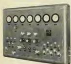
VALVE ACCEPTANCE TEST PANEL FOR PNEUMATIC MISSILE SYSTEM COM PONENT TESTING.
